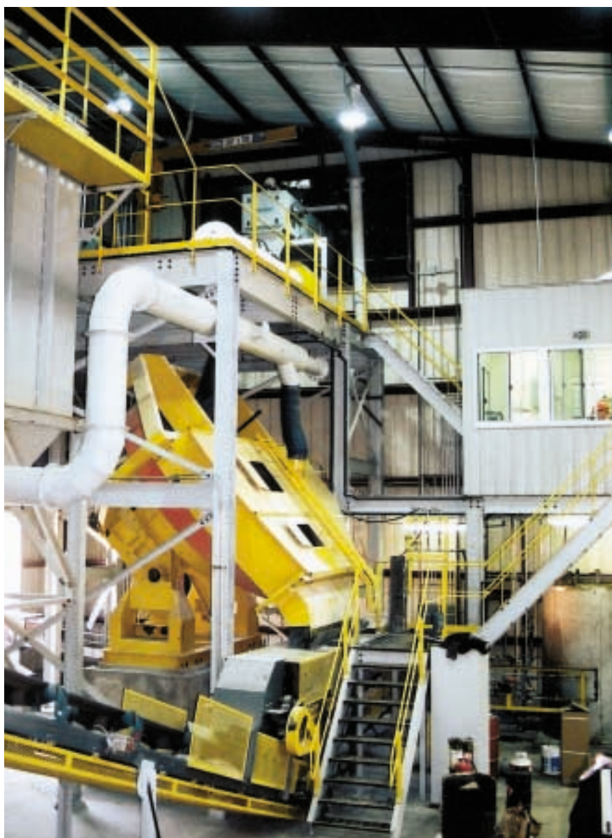
Binder solution continues to mist over the material as the disc pelletizer turns the powdered limestone into limestone pellets that range from 850 to 4,750 microns.
