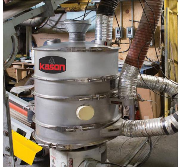
For any pelletizing system, the dryer is specified according to the desired throughput and amount of water to remove from the green pellets. The pilot line's 30" two-deck circular fluid-bed dryer is equipped with a 500,000 BTU/hr (147 kW) heater.
